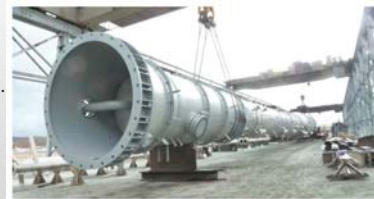
Demethanizer and Cold Separator Designed and built by Eaton Metal Products
